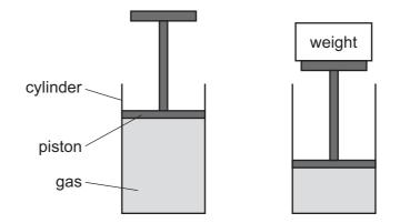
A weight is put on the piston. The volume of gas supporting the piston decreases but the temperature of the gas is unchanged.
