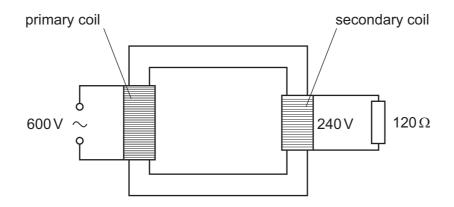
What is the power dissipated in the resistor and the current in the primary coil?
